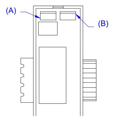
Figure 12: Lynx™ Dual Relay Output Replaceable Fuse Location
