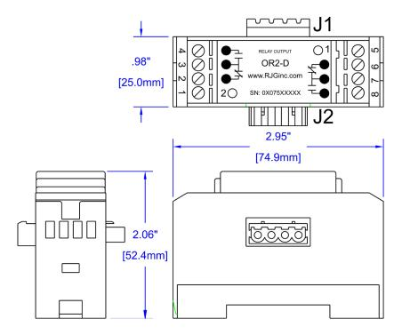
Figure 8: Lynx™ Dual Relay Output Module
