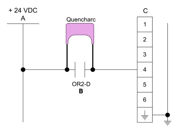
Figure 10: Lynx™ Dual Relay Output Module Robot Interface
