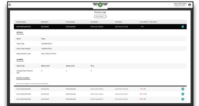
The screenshot shows a 'Process Log' table with columns for Machine Name, Mold Name, Process Name, Job Start, Job End, and End of Batch - Prod Status. Below the table is a 'DETAILS' section with fields for Name, Plant Code, Work Order Number, and Material Batch Code. Below that is an 'ALARMS' section with columns for Alarm Type, Alarm Level, Alarm Limit, and Error. At the bottom is a 'PROCESS CHANGES' section with a table of process changes.
